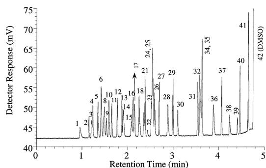
Fig. 2. Separation of commonly used organic solvents.
